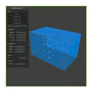
Lastly we have added three sliders to our GUI in order to manipulate the bounding box: length x, length y, and length z. These simple parameters allow us to easily resize the bounding box volume in three dimensions.
